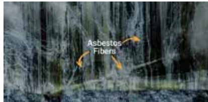
Photo: Close-up image of Canadian chrysotile shows the fibrous composition of the mineral and how easily the fibers can become airborne. Courtesy Asbestorama
