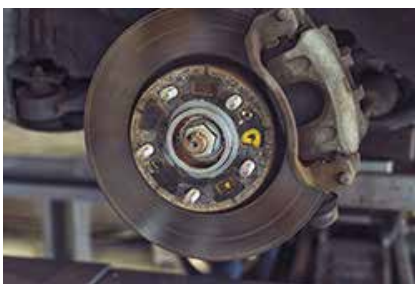
Photo: Older brakes and foreign-made brakes may contain asbestos.
