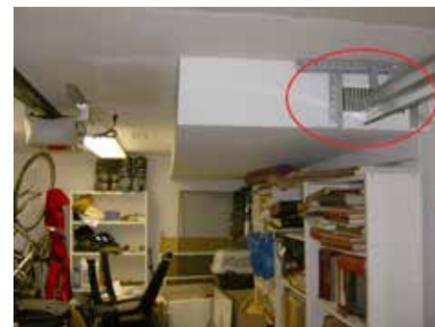
Look carefully inside garages for any supply or return registers – especially where it appears the garage is being used as a workspace.
