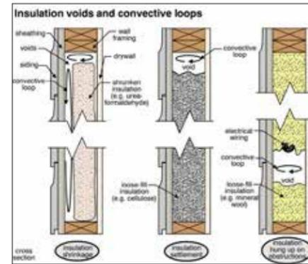
Loose-fill insulation that is blown or poured in can also settle, creating voids at tops of wall cavities, for example. Where insulation is poured or blown into wall cavities, voids may develop if the insulation gets hung up on obstructions partway down the cavity. Voids may also develop in insulations that shrink. Urea-formaldehyde foam insulation sometimes shrank dramatically after it was installed, reducing its R-value.
