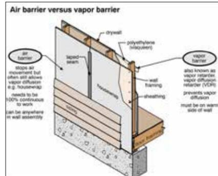
As you can see, a vapor diffusion retarder has fewer functions and is less critical than an air barrier. Let's look at air barriers first.
