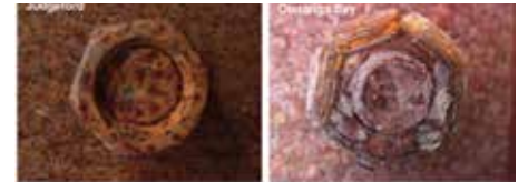
BRANZ Study: Marine Environment Accelerates Corrosion. (left) Bolt/Nut - 3 Years Mild Environment; (right) Bolt/Nut - 3 Years Marine Environment
